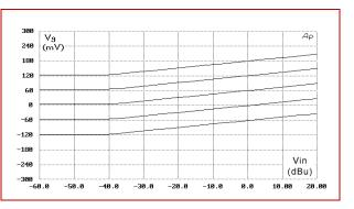
Figure. 4.  $V_G$  vs.  $V_{IN}$  for various GAIN settings.
