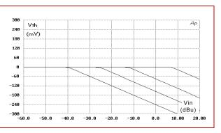
Figure 2. V<sub>TH</sub> vs. VIN for various THRESHOLD settings.
