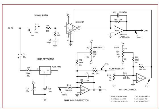
Figure 1. Basic Above-Threshold Compressor/Limiter.
