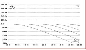
Figure. 7.  $V_{TH}$  vs.  $V_{IN}$  for the Soft-Knee Circuit.
