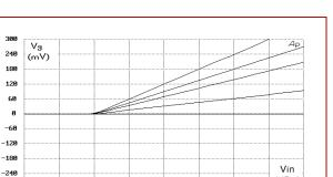
Figure 3. V<sub>G</sub> vs. V<sub>IN</sub> for various COMPRESSION settings.
