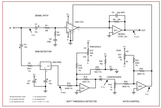
Figure. 6. Basic Soft-Threshold Compressor/Limiter
