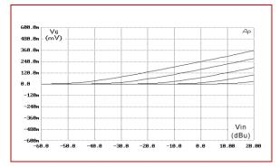
Figure. 8.  $V_G$  vs.  $V_{IN}$  for the Soft-Knee Circuit.
